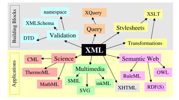
Figure 1. The XML family (adapted from [16])
