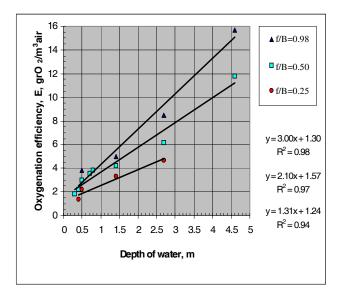
**Figure 7:** Effect of water depth level (h) on oxygenation efficiency (E) at constant air flow rate.
