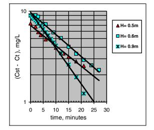
**Figure 4:** Sample of the experimental results showing the variation of  $\log (C_{st} - C_t)$  over time at various water depths.
