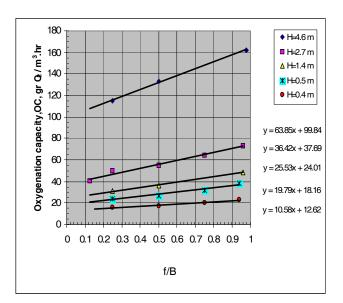
**Figure 6:** Effect of (f/B) ratios on the oxygen transfer capacity (OC) of the system at constant air flow rate.
