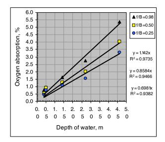
**Figure 9:** Effect level of depth of water (h) on oxygen absorption  $(\delta)$  at constant air flow rate.
