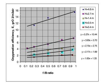
**Figure 8:** Effect of (f/B) ratio on oxygenation efficiency (E) of the system at constant air flow rate.
