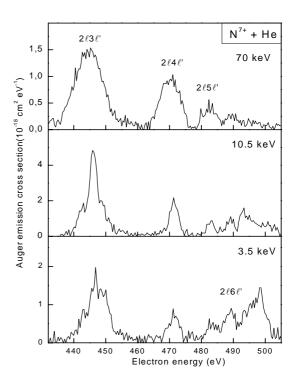
**Figure 2.** High-resolution spectra of *K*-Auger electrons produced in  $C^{6+}$  + He and  $N^{7+}$  + He collisions at a few projectile energies.
