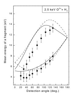
**Figure 9.** Maximum of fragment energy distribution following O<sup>5+</sup> + H<sub>2</sub> collisions at 75 keV and 2.5 keV. Full squares, experimental values; dashes curves, TS2B calculations; solid curves, OS3B calculations.
