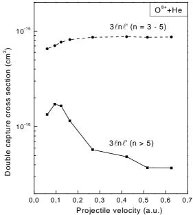
**Figure 5.** DC cross section for populating configurations of quasi equivalent and non equivalent electrons for  $N^{7+}$  + He and  $O^{8+}$  + He collisions as a function of the projectile velocity.
