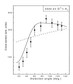
**Figure 10.** Differential cross section for detecting one fragment in 75 keV and 2.5 keV O<sup>5+</sup> + H<sub>2</sub> collisions. Full squares, experimental values; dashes curves, TS2B calculations; solid curves, OS3B calculations.
