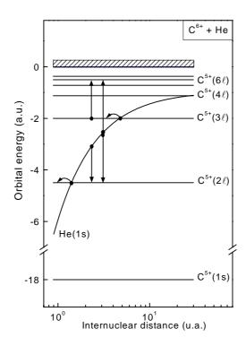
**Figure 1.** Diagram of orbital energies for the system (C-He)<sup>6+</sup>.
