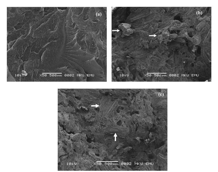
**Figure 4.** SEM micrographs of the a) unfilled recycled HDPE, b) eucalyptus wood residue filled recycled HDPE composites and c) MAPE modified eucalyptus wood residue filled recycled HDPE composites
