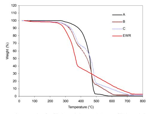
**Figure 1.** TGA thermographs of unfilled recycled HDPE (A), EWR filled recycled HDPE composites (B), EWR filled recycled HDPE composites modified with MAPE coupling agent (C) and eucalyptus wood residue (EWR).
