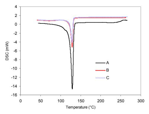
**Figure 3.** DSC thermographs of the recycled HDPE (A), eucalyptus residue filled recycled HDPE composites (B) and eucalyptus wood residue filled recycled HDPE modified with MAPE coupling agent (C).
