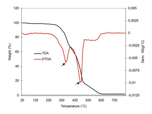
**Figure 2**. TGA and DTGA thermographs of the eucalyptus wood residue filled recycled HDPE composites.
