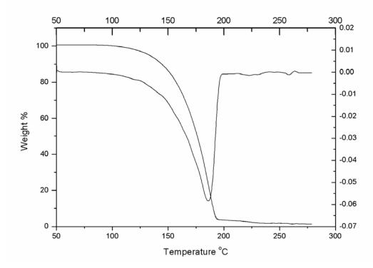
Figures 6 and 7 are the DSC and TG-DTG curves of 2,3-DPX. The curves are similar to those of 2,6-DPX as we can observe two endothermic peaks in Figure 6 and one stage mass loss in Figure 7. In the DSC curve the first endothermic peak temperature is at 92.8 °C, which matches with the literature melting point of 90-93 °C.
