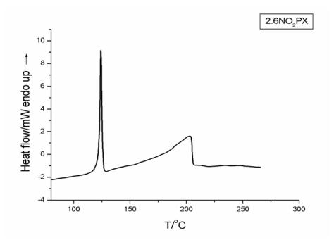
Figure 4. DSC curve of the 2,6-DPX
