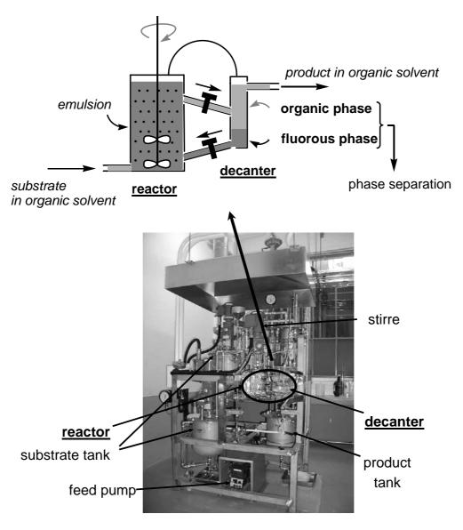
Figure 2. Bench-scale continuous-flow reaction system.
