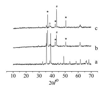
**Figure 8.** XRD spectra of CuO: d) newly prepared; e) used 3 times; peaks with \* are from Cu<sub>2</sub>O, <sup>#</sup> are from Cu.
