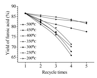
Experiments showed that the calcination temperature greatly affected the recovery of catalyst activity and the optimal temperature was around 250 °C (Figure 9).
