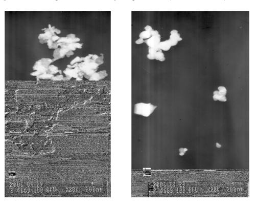
Figure 10. TEM spectra of the catalyst Ag<sub>2</sub>O/CuO; a) used 3 times; b) used 18 times.
