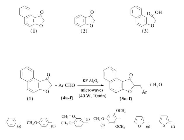
Scheme 2. Condensation under focused microwave irradiation.
