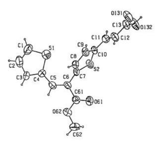
Figure 2. X-Ray structure of 3-{5-[1-methoxycarbonyl-2-(2-thienyl)-ethenyl]-2thienyl}acrylic acid (5) bonded into dimers via H-bonding
