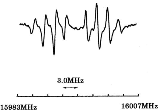
**Figure 5.** Stark pattern of the P(5,4) line in the (2,A, 4) sequence observed with the upper sideband of 9P(40) CO<sub>2</sub> laser line. The horizontal axis is the modulation frequency. The Stark field is dc-bias of 62.5 V/cm with sine-wave modulation of 12.5 V/cm p-p.
