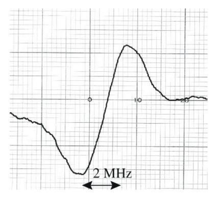
**Figure 3.** Recorder tracing of the microwave transition E,  $l_0 \leftarrow 2_{-1}$  in the ground state at 60531.47 MHz with the infrared transition  $l_{-1}$ ,  $v_{co} = 1 \leftarrow 2_{-1}$ ,  $v_{co} = 0$ . The sample pressure is 167 mTorr. The maximum and the minimum of the signal are separated by 2 MHz in frequency, coming from the microwave frequency modulation.
