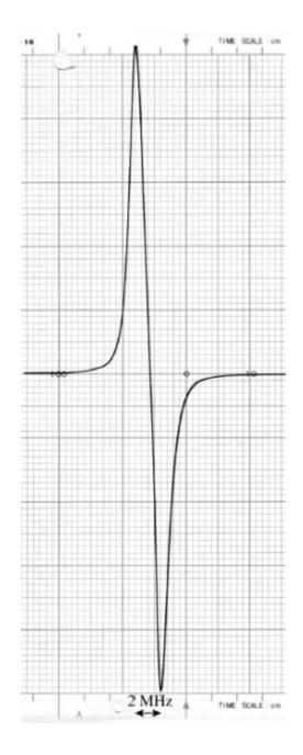
**Figure 1.** Recorder tracing of the microwave transition  $v_{co} = 1$ , E,  $16_2 \leftarrow 16_1$ , of CH<sub>3</sub>OH at 49908.35 MHz with the infrared transition  $16_1$ ,  $v_{co} = 1 \leftarrow 15_1$ ,  $v_{co} = 0$ . The sample pressure is 6 mTorr. The maximum and the minimum of the signal are separated by 2 MHz in frequency, coming from the microwave frequency modulation.
