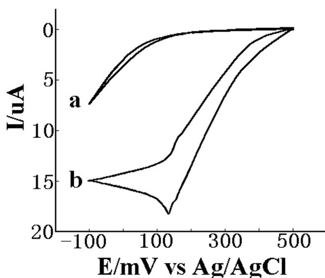
**Figure 2.** Cyclic voltammograms of  $H_2O_2$  recorded by (a) the bare Pt electrode and (b) the PB/Pt electrode.
