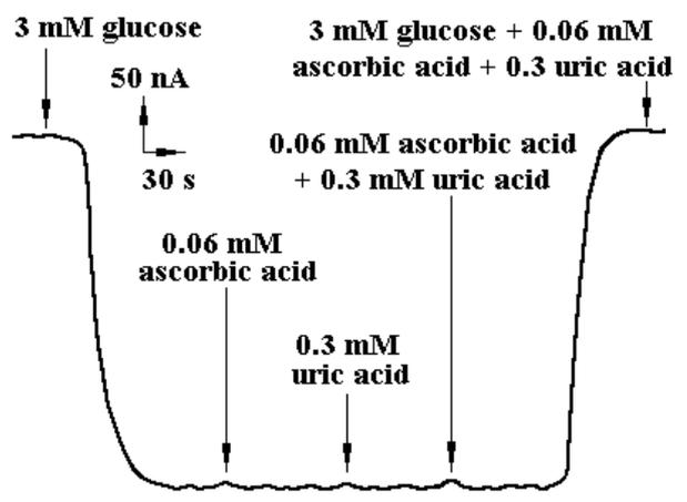
**Figure 8.** Response of the sensor in the presence of ascorbic and uric acids.
