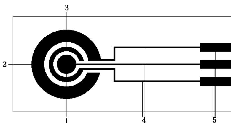
**Figure 1.** Schematic of the chip: 1) WE, 2) CE, 3) Ag/AgCl RE, 4) Conductive lines, 5) Pads.
