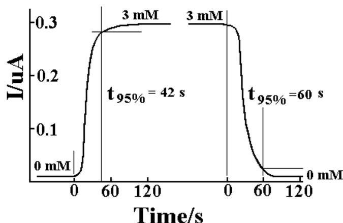
**Figure 6.** The response time curves of the sensor.
