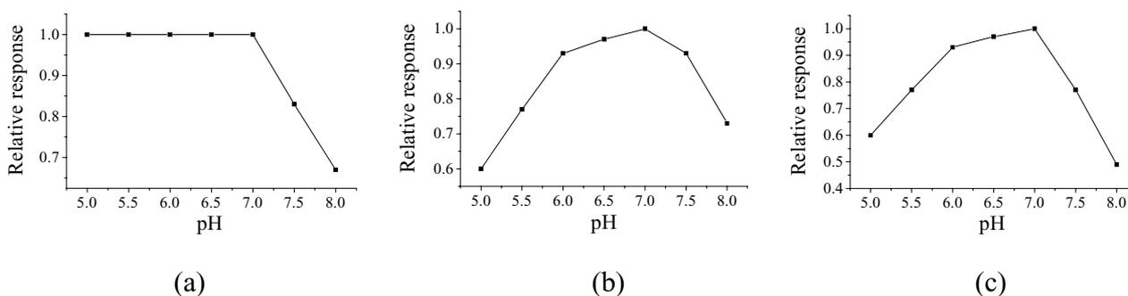
**Figure 4.** Effect of pH on the responses for (a) PB/Pt electrode, (b) GOD/Pt electrode and (c) GOD/PB/Pt electrode.
