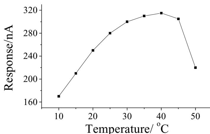
**Figure 5.** Effect of temperature on response current of the sensor.
