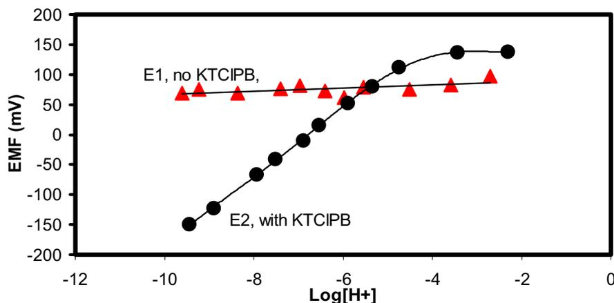
**Figure 1.** The response of hydrogen ion sensor of non-plasticised methacrylic-acrylic membrane to various concentrations of hydrogen ion (0.05 M TrisHCl buffer) in 0.1 M sodium ion. E1: membrane contained only a hydrogen ionophore, E2: Membrane contained both hydrogen ionophore and the lipophilic salt, KTCIPB.
