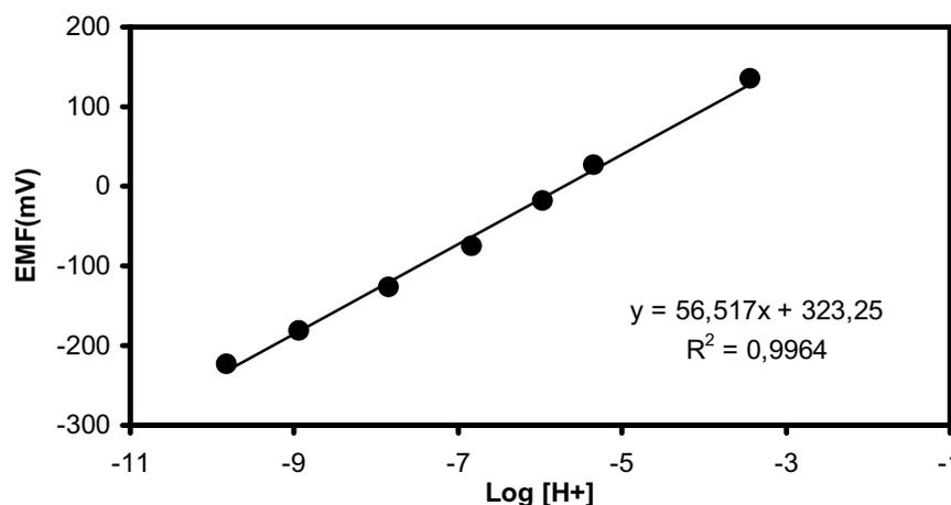
**Figure 2.** The potentiometric response of sensor E2 with a non-plasticised methacrylic-acrylic membrane containing hydrogen ionophore and KTCIPB.
