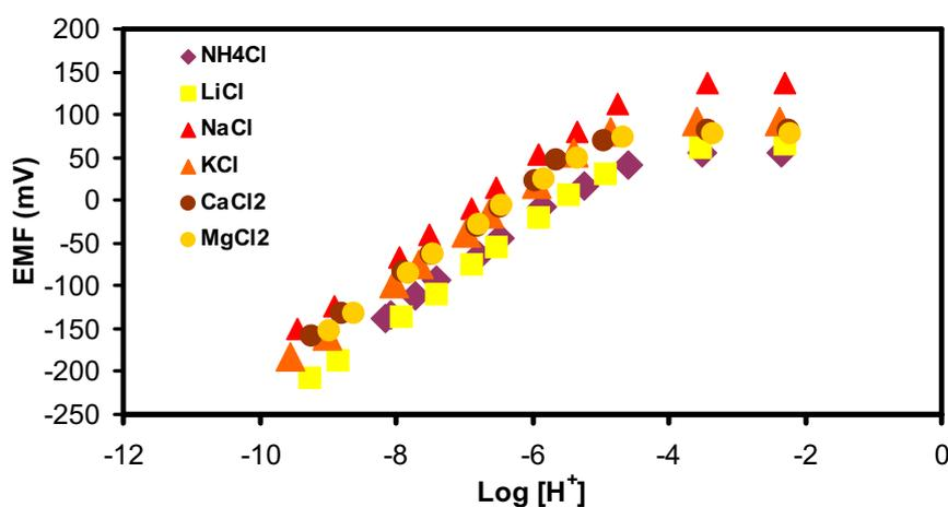
**Figure 3.** The presence of 0.1 M of various cations in the solution did not interfere with the pH response of electrode E2 (From Figure 3).
