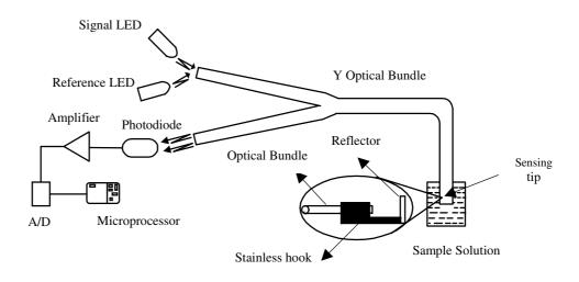
Figure 2. Experimental set-up of the sensing system.
