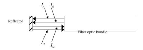
Figure 1. The principle of the double-beam compensation. The sensing tip is dipped into sample solution containing an absorbing substance.
