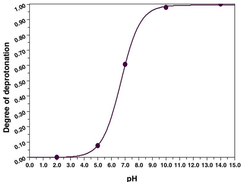
**Figure 3.** The response ( $\alpha$ ) for an optode with a MB28 film exposed to pH 2-14.
