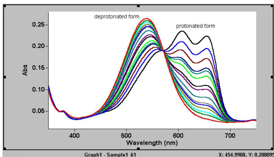
**Figure 2.** The absorption behaviour of a MB28 optode film containing chromoionophore ETH5294 and NaTFPB in 6M of NaOH showing conversion of the initial fully protonated form to the completely deprotonated form.
