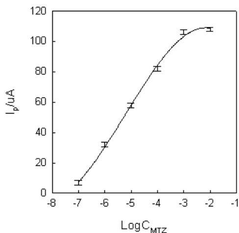
**Figure 5.** Calibration graph for the MTZ sensor obtained with the MTZ sensor incubated in MTZ solutions of different concentrations followed by voltammetric measurements. Operating potential: - 408 mV vs. SCE.
