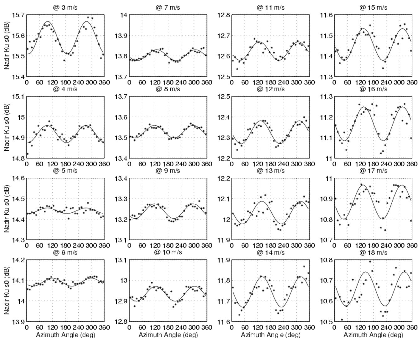
**Figure 1.** Wind direction signal in  $10^\circ$  bins of the Ku-band altimeter radar cross-section for different wind speeds at  $\pm 0.5$  m/s and varying from 3 to 18 m/s. The solid line represents the second-order harmonic fit of form (3).
