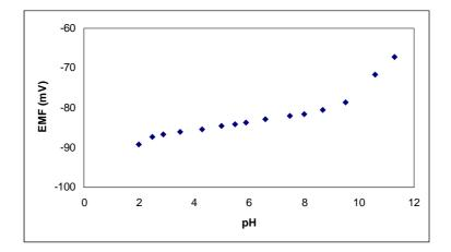
Figure 6. Effect of pH on cell potential.
