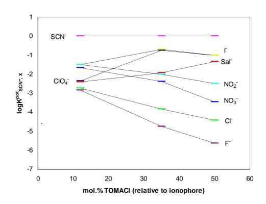
**Figure 3.** Selectivity coefficients,  $\log K_{SCN^-,X^-}^{\text{pot}}$ , for PVC/*o*-NPOE membranes doped with ionophore CoTMeOPP and various concentrations of cationic additive
