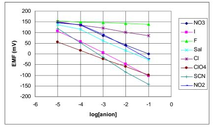
**Figure 5.** Potentiometric anion responses of the electrodes prepared with a membrane having the optimal composition.
