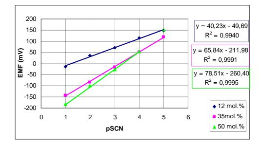
**Figure 4.** Potentiometric responses of membranes containing ionophore CoTMeOPP in PVC/*o*-NPOE matrix to thiocyanate in MES buffer, pH=5.5 and various concentrations of cationic additive.
