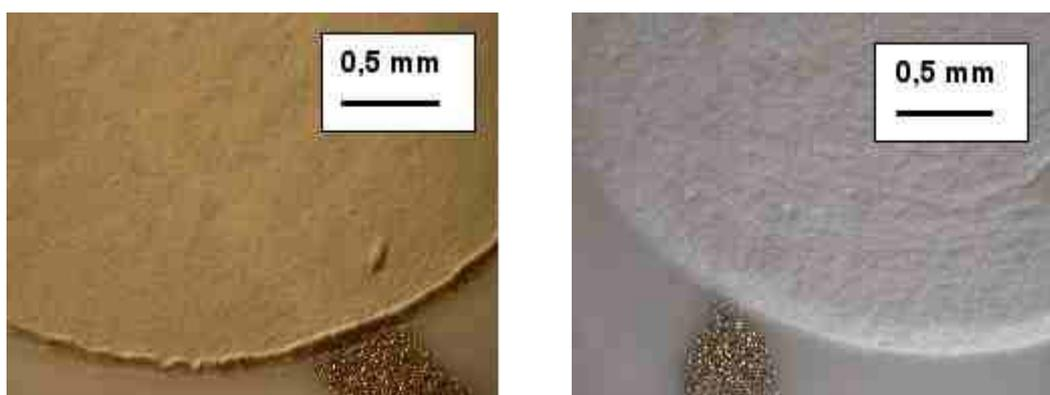
**Figure 3.** Light optical microscope image of a  $\text{WO}_3$  (left) and  $\text{ZrO}_2$  layer (right).
