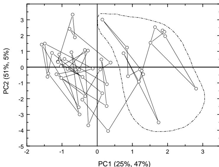
**Figure 12.** PLS-1 score plot of all samples in test mixtures of key odorants containing p-cresolate at pH 8. Samples (15 samples) with high concentrations ( $5 \times 10^{-4}$  -  $10^{-3}$  M) of n-butyrate are surrounded by dashed line. Full cross validation was used and six electrodes were sufficient.
