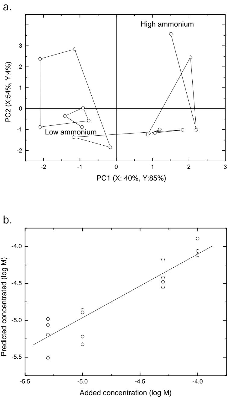
**Figure 6.** a: PLS-1 score plot for 16 samples of ammonium, considering limits of modelling in test mixtures of key odorants containing ammonium at pH 6. b: Calibration curve of identical ammonium samples. PLS-1, full cross validation and two PCs were used and six electrodes were sufficient.
