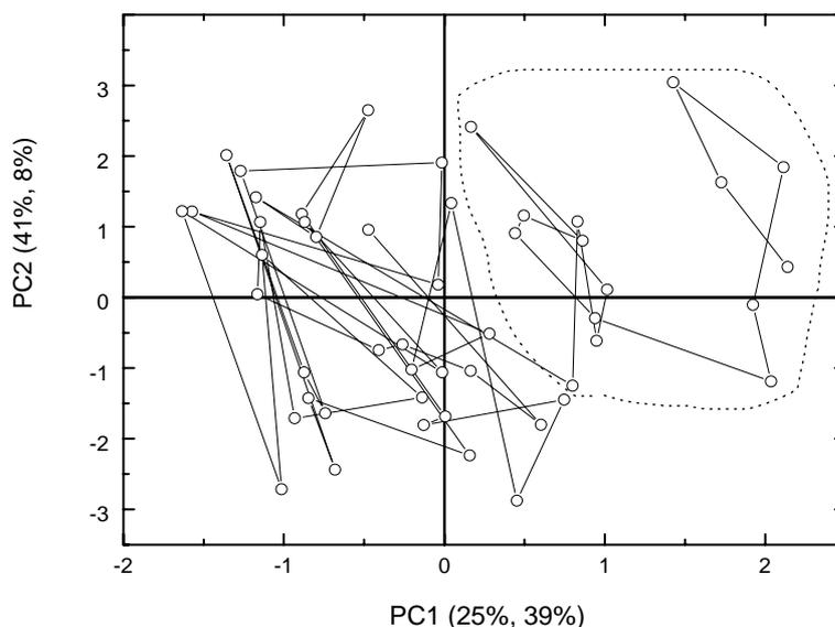
**Figure 9.** PLS-1 score plot of all samples in test mixtures of key odorants containing ammonium at pH 8. Samples (15 samples) with high concentrations ( $5 \times 10^{-4}$  -  $10^{-3}$  M) of n-butyrate are surrounded by dashed line. Full cross validation was used and six electrodes were sufficient.
