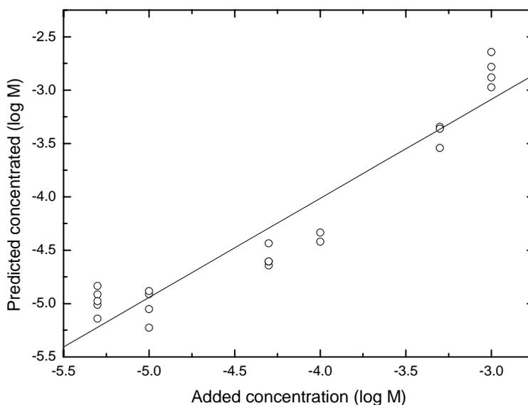
**Figure 3.** Calibration curve of ammonium from  $5 \times 10^{-6}$  to  $10^{-3}$  M at pH 6. PLS-1, full cross validation for 22 samples and two PCs were used and six electrodes were sufficient. Concentration of n-butyrate was below  $10^{-4}$  M.
