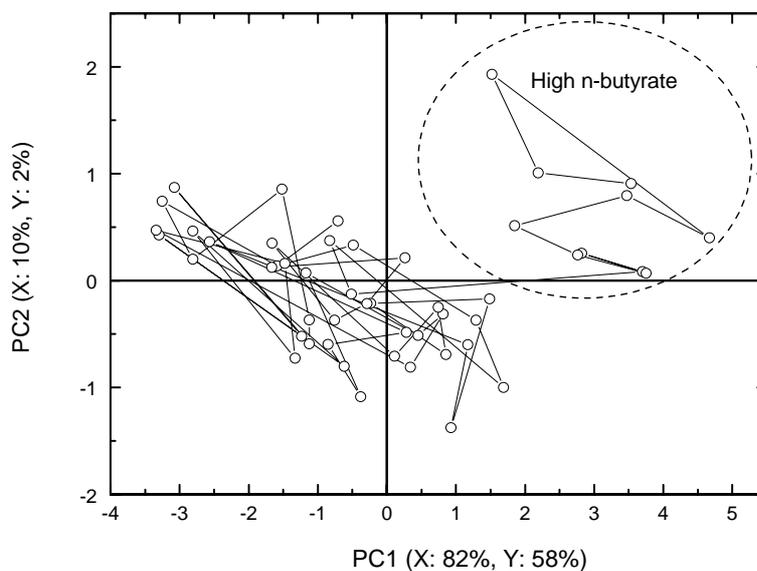
**Figure 7.** PLS-1 score plot of all samples in test mixtures of key odorants containing p-cresolate at pH 6. Samples (10 samples) with high concentrations ( $5 \times 10^{-4}$  -  $10^{-3}$  M) of n-butyrate are surrounded by dashed line. Full cross validation was used and five electrodes were sufficient.
