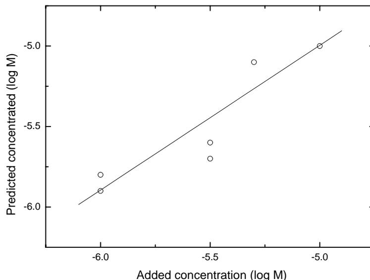
**Figure 11.** Calibration curve (12 samples) of phenolate in test mixtures of key odorants containing ammonium at pH 8. BPNN used 4, 4, 1 nodes.
