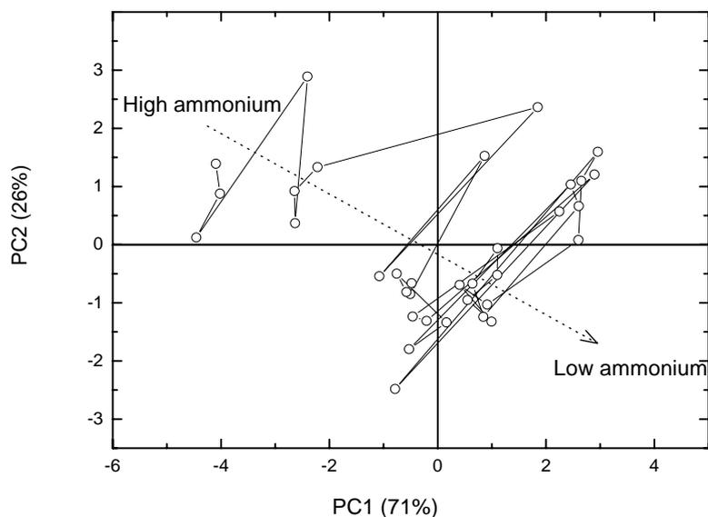
**Figure 2.** PCA score plot of 34 samples in test mixtures of key odorants containing ammonium at pH 6. Concentration of n-butyrate was below  $10^{-4}$  M. Full cross validation was used and six electrodes were sufficient.
