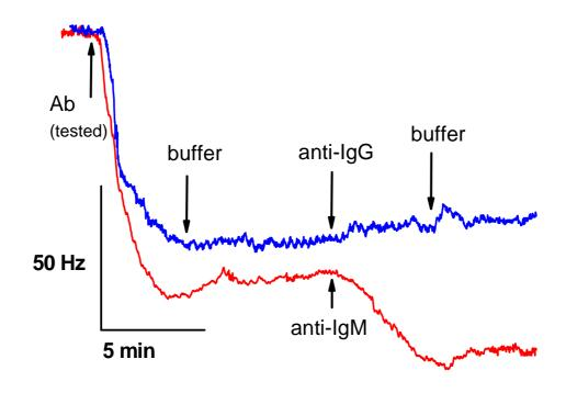
**Fig. 4.** Isotyping of the mAb 4H3B9D3 using the piezoelectric sensor modified with LPS from *F. tularensis*. At first, the tested antibody was allowed to bind on the surface and after washing with buffer, either anti-IgG (blue curve) or anti-IgM (red curve) secondary antibody was injected.
