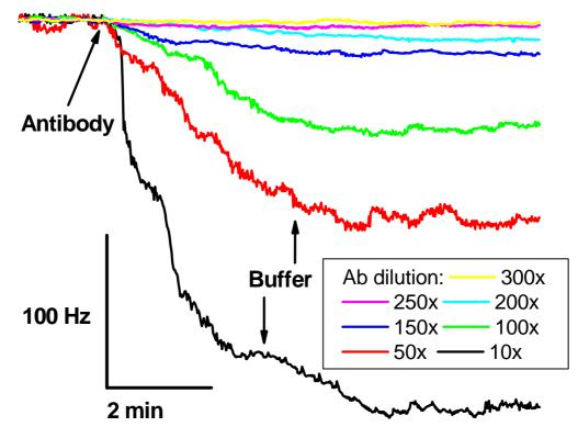
Fig. 5. The influence of the mAb 4H3B9D3 dilution (indicated inside the figure) on the binding response obtained with the piezoelectric sensor modified with the LPS from *F. tularensis*. The sample volume was  $100 \ \mu$ l.
