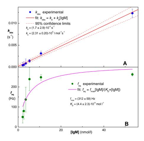
**Fig. 6.** Evaluation of the kinetic parameters for the mAB 4H3B9D3. The binding traces (similar as shown in Fig. 5) were approximated by the eq. 2 and the parameters  $k_{obs}$  (top, blue) and  $f_{eq}$  (bottom, olive) obtained using the non-linear regression are plotted vs. the corresponding molar concentration of the antibody. The dependence of  $k_{obs}$  was linearized (top, red line), the dependence of  $f_{eq}$  was fitted to a hyperbolic equation (bottom, magenta curve).
