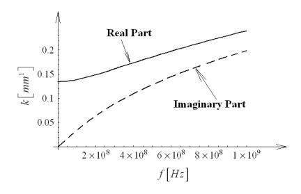
**Figure 8.** Real and imaginary parts of the wave vector, k, assuming  $\mu_a = 0.006 \ mm^{-1}$  and  $\mu_s = 1.0 \ mm^{-1}$ .
