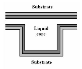
Figure 15. Hollow waveguides cross section.
