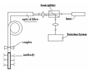
**Figure 5.** Typical fluorescence-based photonic sensor.
