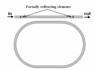
**Figure 26.** Micro racetrack resonator biosensor with sensitivity enhanced by introducing two partially reflecting elements.
