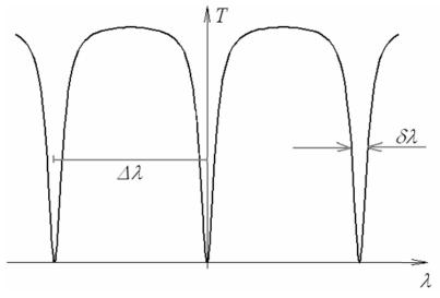
Figure 24. Typical transmittivity spectrum of a micro resonator.
