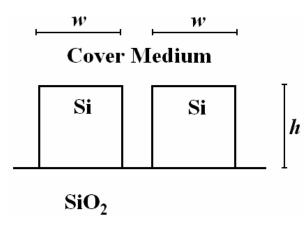
Figure 20. SOI slot waveguide structure.
