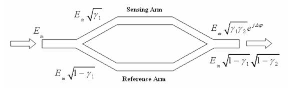
Figure 10. Mach-Zehnder interferometer architecture.
