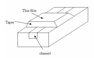
**Figure 13.** Schematic diagram of a channel-planar composite optical waveguide.
