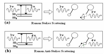
Figure 6. Raman scattering mechanisms.
