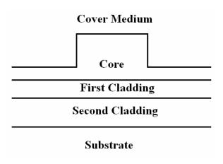
Figure 14. ARROW waveguide structure.
