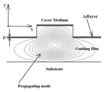
**Figure 9**. Effective index change in integrated optical sensors.
