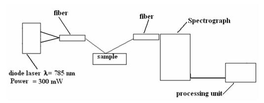
**Figure 7.** Typical apparatus for Raman spectroscopy.
