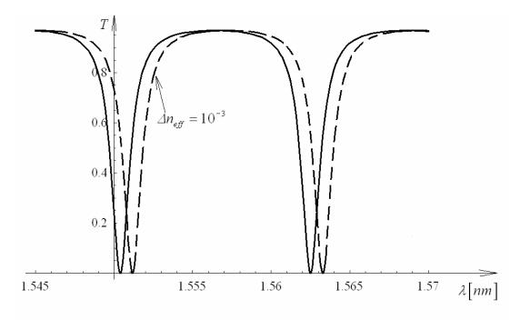
**Figure 25.** Transmittivity spectrum of a micro resonator having  $L_t = 100 \, \mu m$ , A = 0.99,  $r^2 = 0.7$ ,  $t^2 = 0.3$  and  $n_{eff} = 2$  and spectrum translation due to a shift in effective index equal to  $10^{-3}$ .
