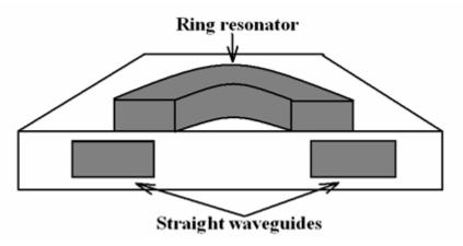
Figure 27. Vertical coupling between microring and straight waveguides.
