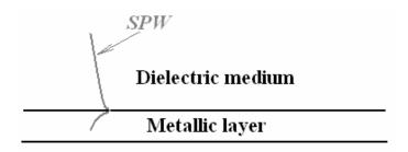
Figure 17. Planar structure in which SPW propagates.
