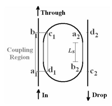
Figure 23. Resonator race-track structure schematic representation.
