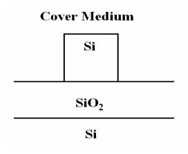
Figure 19. Si-wire waveguide structure.
