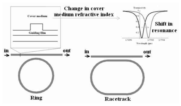
**Figure 22.** Micro cavity-based architectures for integrated optical sensors.
