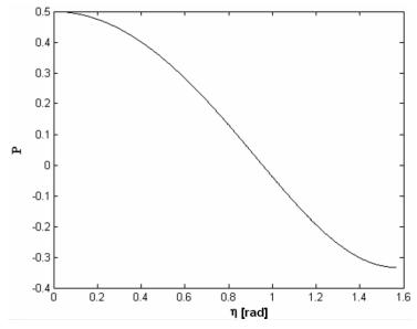
**Figure 4.** Degree of polarization versus  $\eta$ . If  $\eta = 0^{\circ}$ , absorption and emission vectors are parallel and P = 0.5. If  $\eta = 90^{\circ}$ , absorption and emission vectors are perpendicular and P = -0.33.
