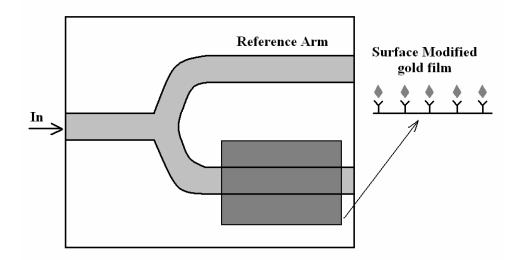
**Figure 16.** Integrated optical biosensor exploiting the SPR scheme.
