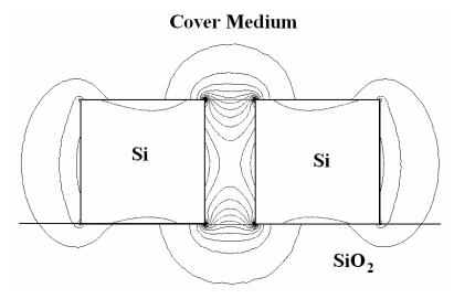
Figure 21. Quasi-TE mode profile in silicon slot waveguide.
