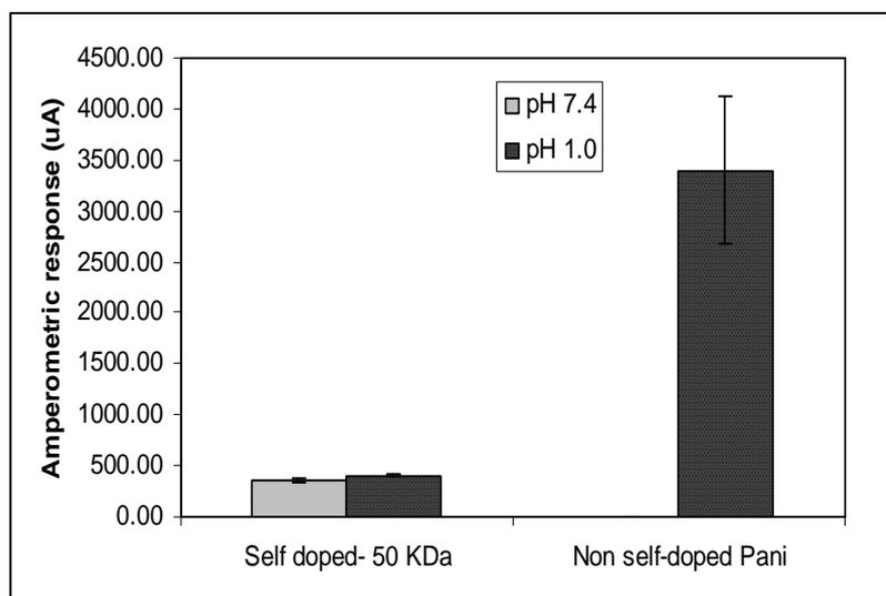
**Figure 6.** Amperometric responses of ITO substrates coated with non-self doped Pani and 50 KDa self doped Pani in two pH controlled electrolytes.
