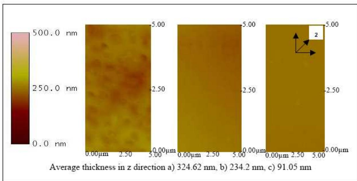
**Figure 10.** Atomic force microscopy images of a) ITO glass treated with (NH<sub>4</sub>OH) and spin coated with 65KDa, b) 50KDa, c) 20KDa Pani.
