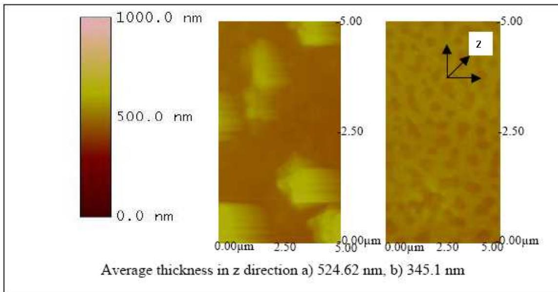
**Figure 12.** Atomic force microscopy images of a) ITO-Pani biosensor (65KDa) tested with a)  $10^6$  CCID/ml and b)  $10^4$  CCID/ml of bovine viral diarrhea virus (BVDV).
