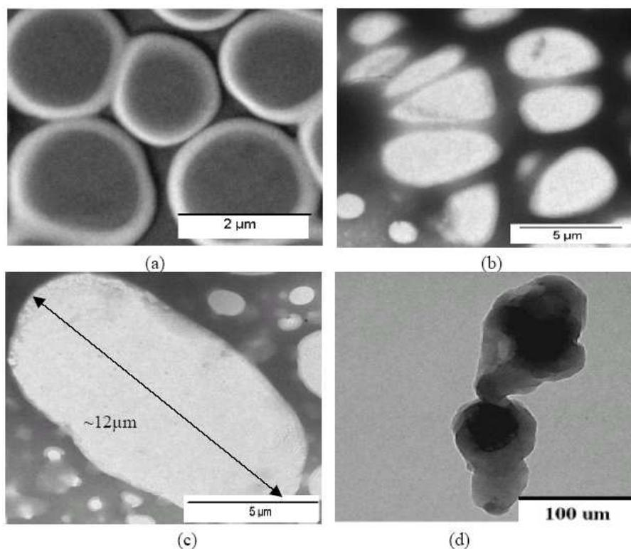
**Figure 3.** Transmission electron microscopy images of a) 20 KDa, b) 50 KDa, and c) 65 KDa self doped Pani, and d) non-self doped Pani.
