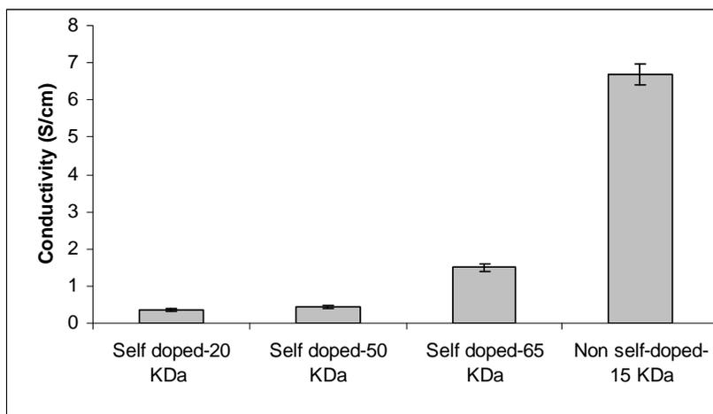
**Figure 2.** Conductivity of polyaniline compounds.
