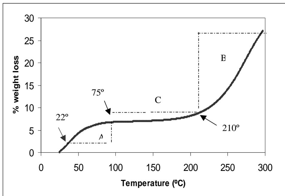
**Figure 5.** Percent of weight loss of 65 KDa Pani in varying temperatures.
