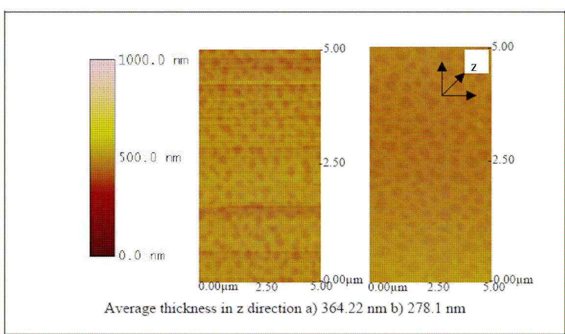
**Figure 13.** Atomic force microscopy images of a) ITO-Pani biosensor (50KDa) tested with a)  $10^6$ CCID/ml and b)  $10^4$ CCID/ml of bovine viral diarrhea virus (BVDV).
