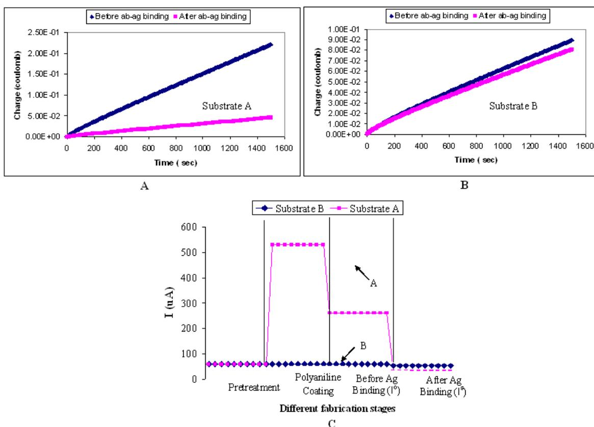
**Figure 15.** Current-versus-time response of A) substrate A (ITO biosensor spin-coated with self-doped Pani and B) substrate B (ITO biosensor without Pani coating). Amperometric responses of both substrates at every fabrication stage (C).
