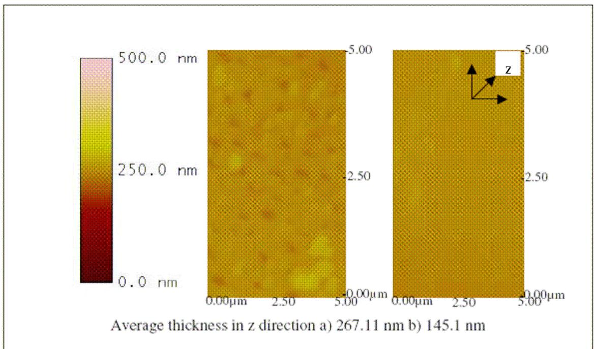
**Figure 14.** Atomic force microscopy images of a) ITO-Pani biosensor (20KDa) tested with a)  $10^6$ CCID/ml and b)  $10^4$ CCID/ml of bovine viral diarrhea virus (BVDV).
