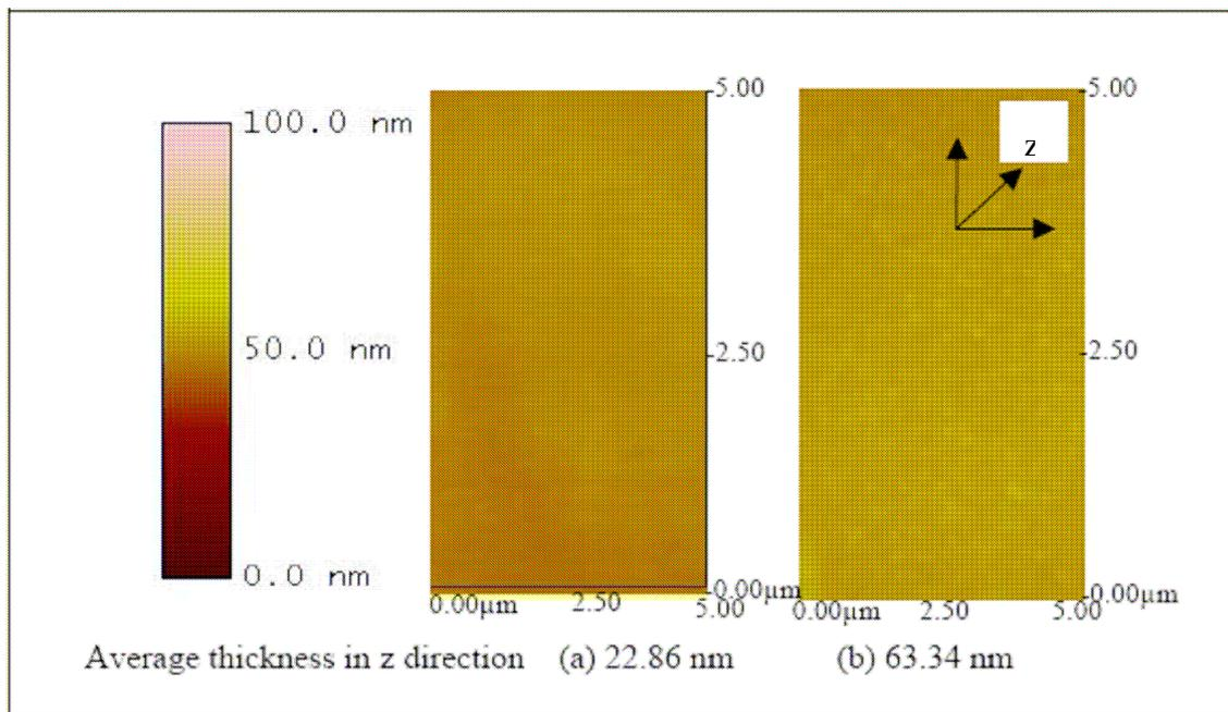
**Figure 9.** Atomic force microscopy images of a) untreated ITO glass and b) ITO glass treated with ammonium hydroxide (NH<sub>4</sub>OH).
