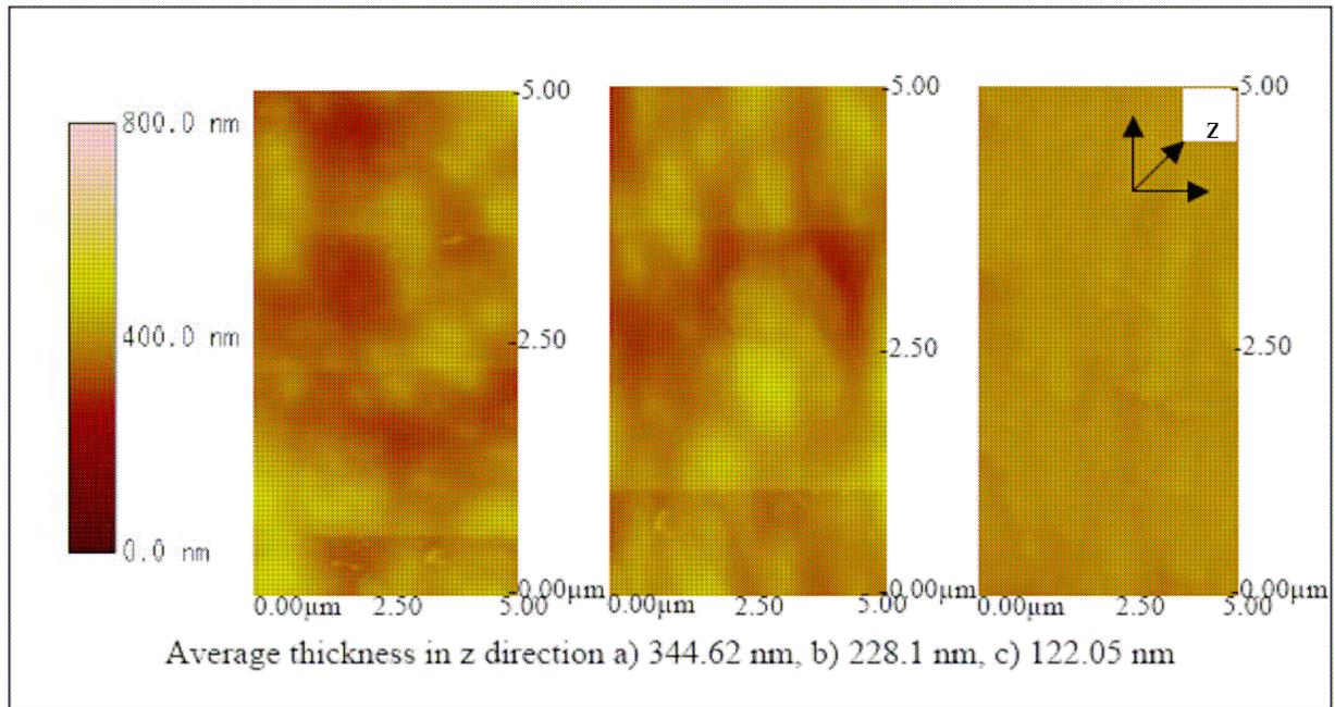
**Figure 11.** Atomic force microscopy images of a) ITO glass spin coated with Pani (65KDa) + antibody, b) Pani (50 KDa) + antibody, and c) Pani (20 KDa) + antibody.
