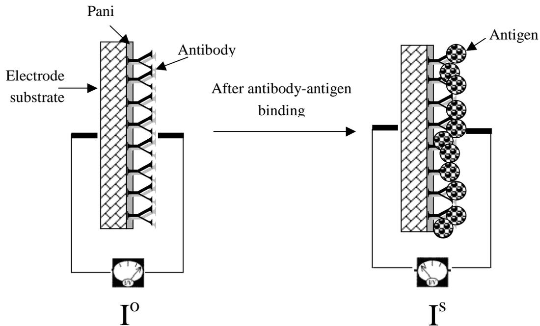
**Figure 7.** Schematic of an ITO-Pani biosensor before and after antibody-antigen binding.
