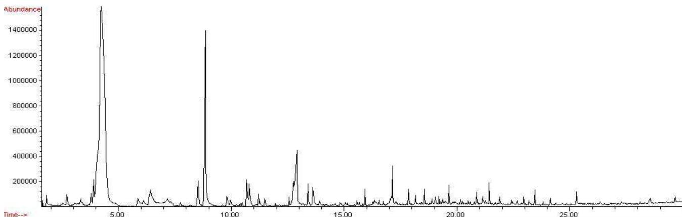
**Figure 4.** Chromatogram of *Penicillium chrysogenum*, CW/DVB, 18 hour exposure.
