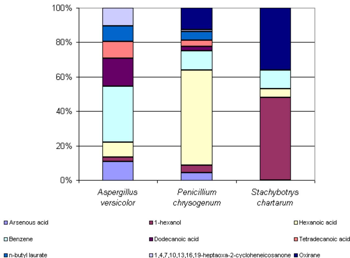
**Figure 6.** Percent peak areas of common compounds found in headspaces of *Aspergillus versicolor*, *Penicillium chrysogenum*, and *Stachybotrys chartarum*, CW/DVB, 18 hour exposures
