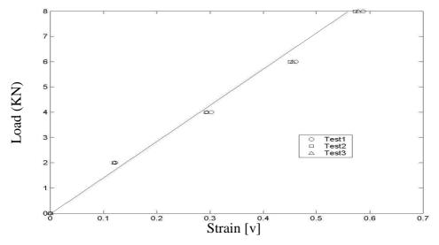
Figure 11. Illustration of the repeatability of the sensor.
