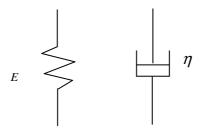
**Figure 4.** Spring and dashpot model.
