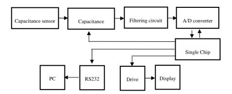
Figure 2. Block diagram of measuring circuit.
