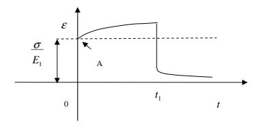
**Figure 6.** Strain curve for Maxwell-Kelvin model.
