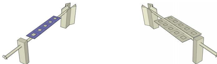
**Figure 3.** Tilting variants: the axial type (left) and the wing type (right).
