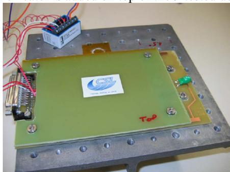
c) The top board is fixed to press the heaters on the devices
