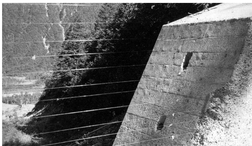
Photocells and infrared photobeam sensors can be utilized as a tool to detect debris flows [11]. The flowing mass interrupts the beams emitted by the sensors, making it possible to detect the passage of the wave. If several sensors are installed at different heights at the same cross-section, it is also possible to approximately measure the peak flow stage.
