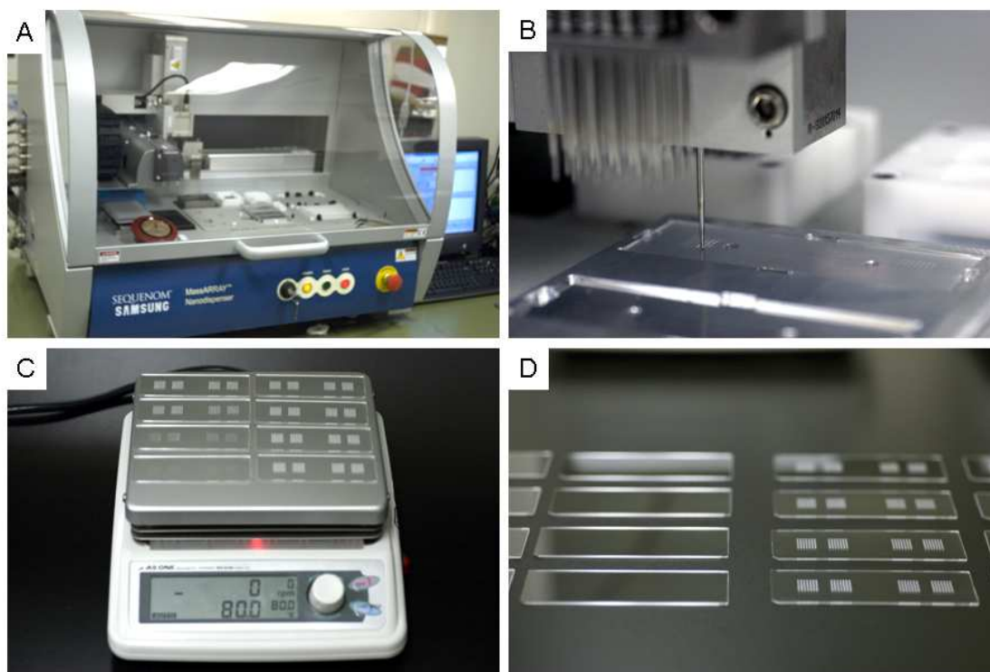
Figure 4. Post spotting processes in preparation of visible genotype sensor array. A: Attaching a Multiwell GeneFrame onto each plastic base. B: Simultaneous handling of multiple plastic bases. C: Masking unspotted surface of plastic bases by soaking in 1 x S-BIO blocking solution. D: Removal of surface solution by centrifugation.
