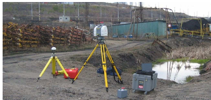
Figure 2. The 3D laser scanner Leica HDS3000 making point cloud acquisition for a slope area on the left, and for the temporary storage place on the right.
