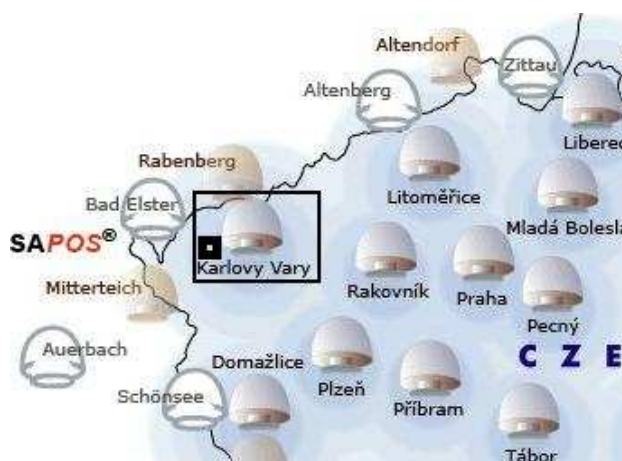
Figure 6. The local network of the GPS reference stations (CZEPOS) in the Czech Republic.
