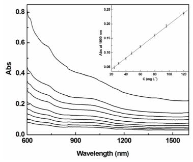
Figure 3. Absorption spectra of SWNT–SnDPP nanohybrid in room temperature THF at different concentrations (from top to bottom: saturated solution, 120, 96, 80, 60, 48, 40, 30 and 24 mg L<sup>-1</sup>). Inset shows the linear relationship of the absorption at 1000 nm versus concentration; slope = 0.002, R = 0.9997.
