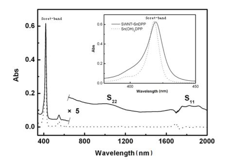
**Figure 5.** UV-Vis-NIR absorption spectra of  $Sn(OH)_2DPP$  (dotted line) and SWNT–SnDPP (solid line) in THF at room temperature ( $C_{porphyrin} = 1.1 \times 10^{-5} \text{ mol } \text{L}^{-1}$ , 25 °C). The inset shows the enlarged Soret-band region.
