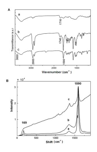
Figure 2. (A) FT-IR spectra of: SWNTs (a), SWNT–SnDPP (b) and Sn(OH)<sub>2</sub>DPP (c). All IR samples are prepared as pellets by using spectroscopic grade KBr at room temperature. (B) Raman spectra of SWNTs (a) SWNT–SnDPP after TGA treatment in nitrogen, 5 °C/min (b) and SWNT–SnDPP (c). Raman spectra are measured at room temperature with the 514.5 nm line of an Ar ion laser as the excitation source.
