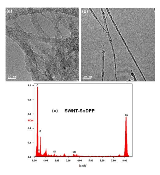
Figure 1. TEM images of purified SWNTs dispersed in DMF via sonication for 30 minutes (a), SWNT–SnDPP dispersed in THF via sonication for 1 minute (b) and EDS analysis of SWNT–SnDPP (c). Measurements performed at room temperature.
