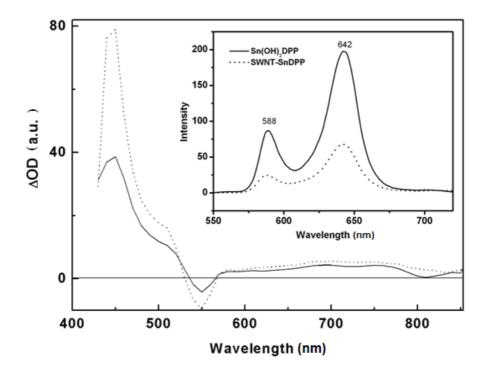
**Figure 6.** Differential absorption spectrum obtained upon nanosecond flash photolysis (532 nm) of SWNT–SnDPP (dotted line) and Sn(OH)<sub>2</sub>DPP (solid line) in argon saturated THF at room temperature with a 50 ns time delay. Inset shows the fluorescence spectra of Sn(OH)<sub>2</sub>DPP and SWNT–SnDPP in THF ( $C_{porphyrin} = 1.1 \times 10^{-5} \text{ mol L}^{-1}$ ) at room temperature.
