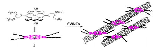
Scheme 1. Schematic view of the Sn(IV) porphyrin (1) functionalized SWNTs.
