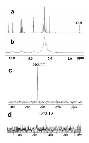
**Figure 4.** NMR (CDCl<sub>3</sub>, 300 MHz, room temperature): <sup>1</sup>H NMR spectra: (a) Sn(OH)<sub>2</sub>DPP, (b) SWNT–SnDPP; <sup>119</sup>Sn NMR spectra: (c) Sn(OH)<sub>2</sub>DPP, (d) SWNT–SnDPP.
