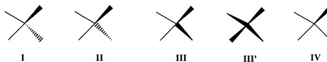
FIGURE 2 Two ways (**I** and **II**) of solid wedge and broken wedge representation most frequently seen in the literature. A first proposal [1] advocated the use of only the solid wedge (**III** or **III'**). Here, we show that a single solid wedge is sufficient to represent configuration at quadrivalent chiral centers (**IV**)
