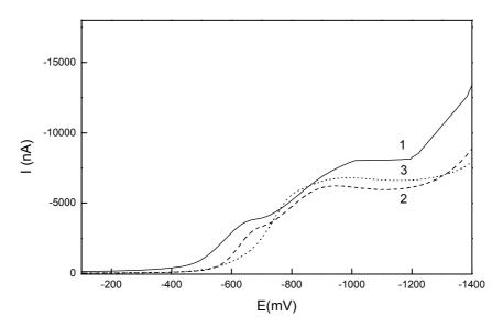
**Figure 5.** Selected LS voltammograms of 1-NP ( $c=1.10^{-4}$  mol.L<sup>-1</sup>) at GCPE in mixture of a BR buffer : MeOH (1:9 v/v) with buffer pH 3 (1), 5 (2) and 8 (3).
