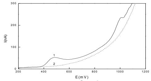
**Figure 3.** Influence of the  $t_{acc}$  for AAV of 2.10<sup>-7</sup> mol.L<sup>-1</sup> 1-AP in stirred solution of a BR buffer pH 2 : MeOH (9:1 v/v),  $E_{acc} = 200$  mV.
