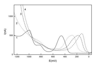
**Figure 2.** Selected DP voltammograms of 1-AP ( $c=1.10^{-4} \text{ mol.L}^{-1}$ ) at GCPE in a mixture of BR buffer : MeOH (9:1) at buffer pH 2(1), 6 (2), (3) 10, 12 (4).
