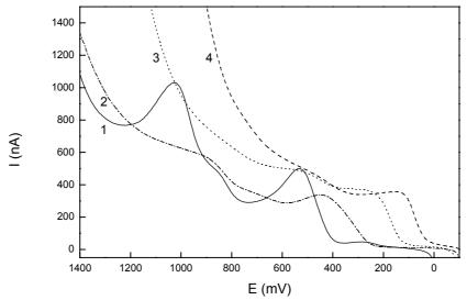
**Figure 1.** Selected LS voltammograms of 1-AP ( $c=1.10^{-4}$  mol.L<sup>-1</sup>) at GCPE in mixture of BR buffer : MeOH (9:1) at buffer pH 2 (1), 6 (2), 10 (3), 12 (4).
