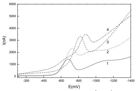
**Figure 6.** Selected DP voltammograms of 1-NP ( $c=1.10^{-4}$  mol.L<sup>-1</sup>) at GCPE in mixture of a BR buffer : MeOH (1:9 v/v) mixture with buffer pH 3 (1) , 5 (2), 8 (3) and 12 (4).
