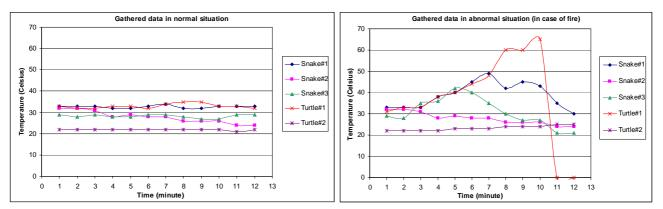
Figure 7. Data gathered from MBSs under both normal and abnormal (fire) conditions.
