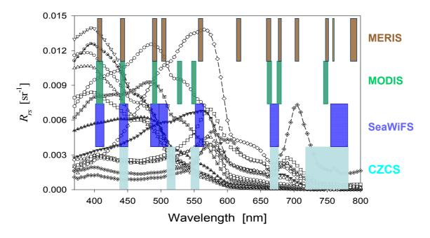
Ideally, to maximize the potential of observing properties of aquatic environments and their temporal and spatial changes, it is best to have a sensor capable of collecting signals with a continuous spectrum. After consideration of data flow, processing, and storage as well as signal-to-noise ratios, satellite sensors commonly have a few bands in the visible and near-IR domain (IOCCG 1998). For
