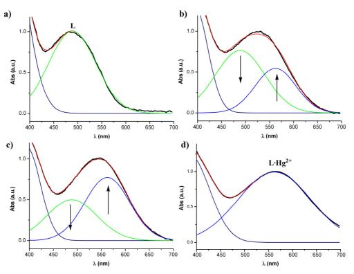
**Figure 3**. Deconvolution of the observed UV-Vis band in two Gaussian bands after soaking the cellulose paper into solution of increasing concentration of mercury ions: a) before soaking and after soaking with b)  $7.5 \cdot 10^{-4}$  M, c)  $2.5 \cdot 10^{-3}$  M, and d)  $1.0 \cdot 10^{-2}$  M of Hg<sup>2+</sup> in acetonitrile.
