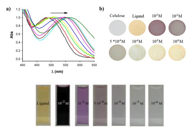
Figure 2. a) Normalized reflectance UV-Vis spectra of the cellulose indicator papers upon dipping onto increasing concentration of Hg(ClO<sub>4</sub>)<sub>2</sub> in acetonitrile. b): "Naked-eye" detection of different concentations of Hg<sup>2+</sup> cation using the cellulose indicator papers. c) Colour changes of azine 1 with different concentration of Hg<sup>2+</sup> in CH<sub>3</sub>CN/H<sub>2</sub>O (7:3, v/v)
