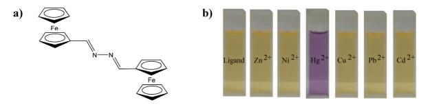
**Figure 1**. a) Highly selective and chromogenic mercury sensor based in a 1,4-disubstituted azine bearing two ferrocene groups. b) Colour change due to binding of **1** in CH<sub>3</sub>CN/H<sub>2</sub>O (7/3, v/v) (c = 1 x  $10^{-3}$  M) with Hg<sup>2+</sup>in comparison with other divalent metal cations.
