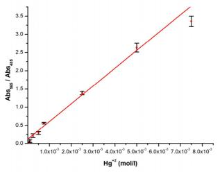
**Figure 4**. Calibration curve of the responses of the cellulose paper with **1** by fitting the area ratio data of the deconvoluted Gaussian bands (see Fig 3) with maxima at these two wavelengths -
